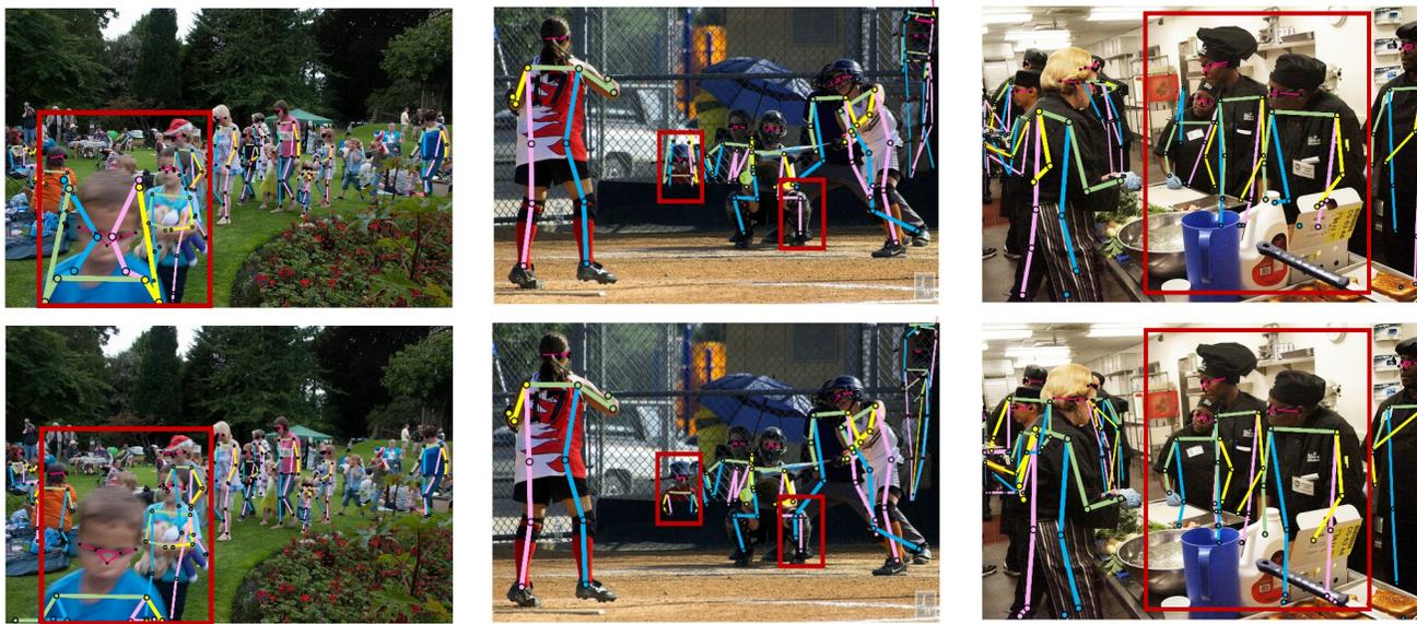
Figure 4. Qualitative results of naive transformer (first row) and our visibility-aware transformer (second row) for keypoints reasoning. We use red squares to highlight our improved prediction qualities when faced with strong occlusion.
